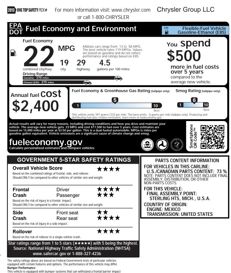
This vehicle is equipped with bumper systems that can withstand a frontal barrier impact speed of 2.5 miles per hour and a rear barrier impact speed of 2.5 miles per hour with no more damage than allowed by the Federal bumper standard. The Federal bumper standard allows damage to the bumpers and attaching hardware and specifies barrier tests to be conducted at 2.5 miles per hour.
