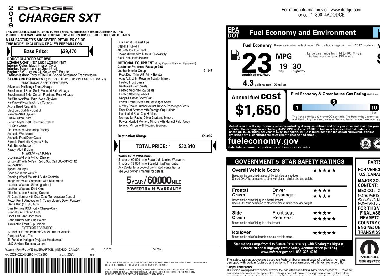
This vehicle is equipped with bumper systems that can with stand a frontal barrier impact speed of 2.5 miles per hour and a rear barrier impact speed of 2.5 miles per hour with no more damage than allowed by the Federal bumper standard. The Federal bumper standard allows damage to the bumpers and attaching hardware and specifies barrier tests to be conducted at 2.5 miles per hour.
