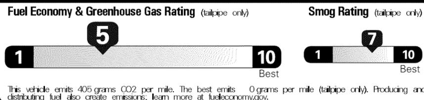
Actual results will vary for many reasons, including driving conditions and how you drive and maintain your vehicle. The average new vehicle gets 26 MPG and costs \$7,000 to fuel over 5 years. Cost estimates are based on 15,000 miles per year at \$2.45 per gallon. MPGe is miles per gasoline gallon equivalent. Vehicle emissions are a significant cause of climate change and smog.
