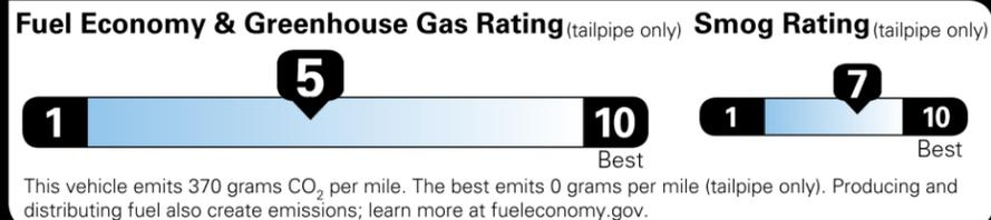
Actual results will vary for many reasons, including driving conditions and how you drive and maintain your vehicle. The average new vehicle gets 28 MPG and costs \$9,750 to fuel over 5 years. Cost estimates are based on 15,000 miles per year at \$4.30 per gallon. MPGe is miles per gasoline gallon equivalent. Vehicle emissions are a significant cause of climate change and smog.
