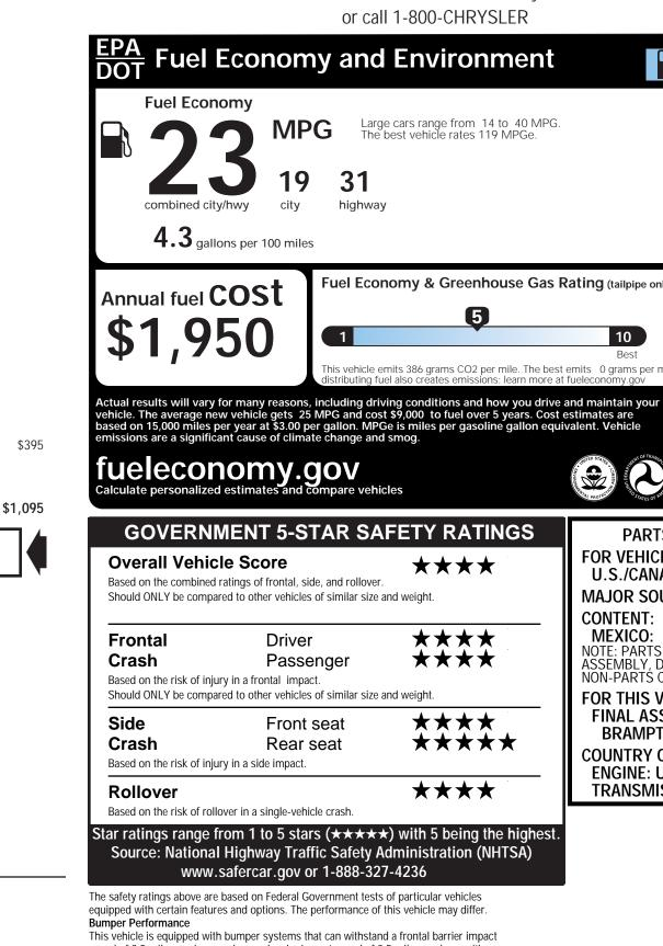
This vehicle is equipped with bumper systems that can withstand a frontal barrier impact speed of 2.5 miles per hour and a rear barrier impact speed of 2.5 miles per hour with no more damage than allowed by the Federal bumper standard. The Federal bumper standard allows damage to the bumpers and attaching hardware and specifies barrier tests to be conducted at 2.5 miles per hour.
