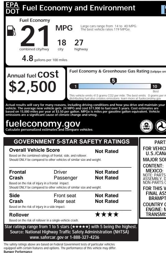
This vehicle is equipped with bumper systems that can withstand a frontal barrier impact speed of 2.5 miles per hour and a rear barrier impact speed of 2.5 miles per hour with no more damage than allowed by the Federal bumper standard. The Federal bumper standard allows damage to the bumpers and attaching hardware and specifies barrier tests to be conducted at 2.5 miles per hour.
